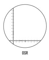
The OSR reticle is designed to maximise field of view at high magnification, whilst allowing the spotter to quickly and efficiently call corrections to the shooter. 1/10th MRAD measuring bars allow for precise range estimation for targets of known size.
