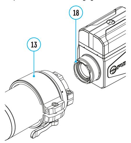
**1.** Remove the protective cover from the eyepiece of the thermal imaging module.
