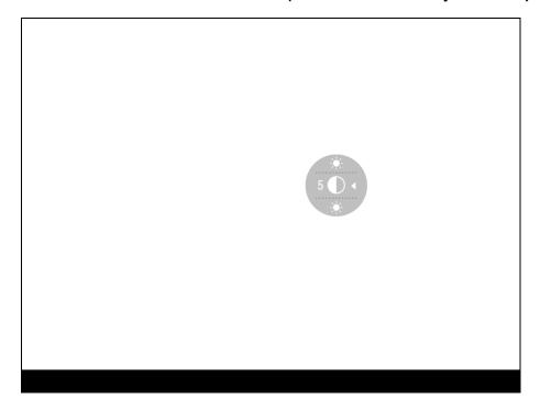
Contrast — press the UP (5)/DOWN (7) buttons to change the display contrast value from 0 to 20.
