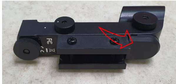
Figure 5: Non-compliant finderscope with cap that can be removed by hand.
