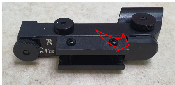
Figure 1: Non-compliant finderscope with battery compartment that can be opened by hand.
