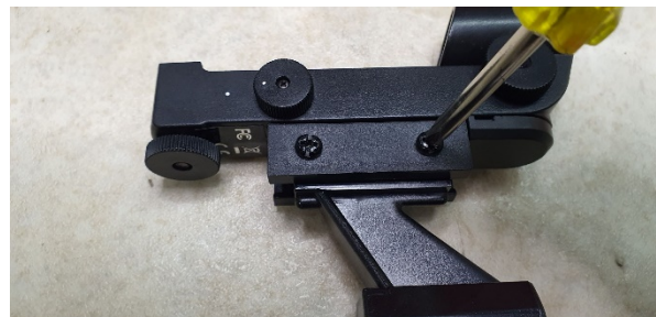
Figure 7: Loosen screws to remove mounting shoe, attach shoe to new finderscope.
